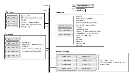
Fig. 3 OpenStack architecture, logical design, nodes, network, and services.
