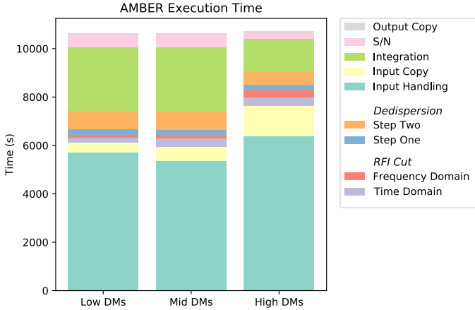
Fig. 16. Break down of functions for the three AMBER instances that run on each CB/compute node. Shown are the various total execution times per function, that together ran real-time on the 3 h observation.
